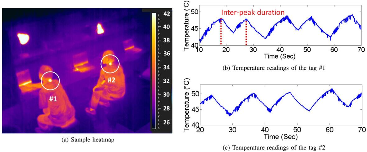
Figure 1: The sample heatmap and temperature readings for tags #1 and #2. Two tags (two glowing dots indicated by the white circles) were worn by two different occupants (using their notebook PCs) in (a). The human identities are encoded in the combinations of various inter-peak durations modulated in the corresponding temperature readings of (b) and (c).
