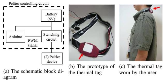
Figure 4: The schematic block diagram and prototype of a thermal tag. The Peltier controlling circuit is wired to the Peltier device (marked by red arrow) along the black stripe as shown in (b). This tag is worn by a user with the Peltier device placed on his neck in (c).
