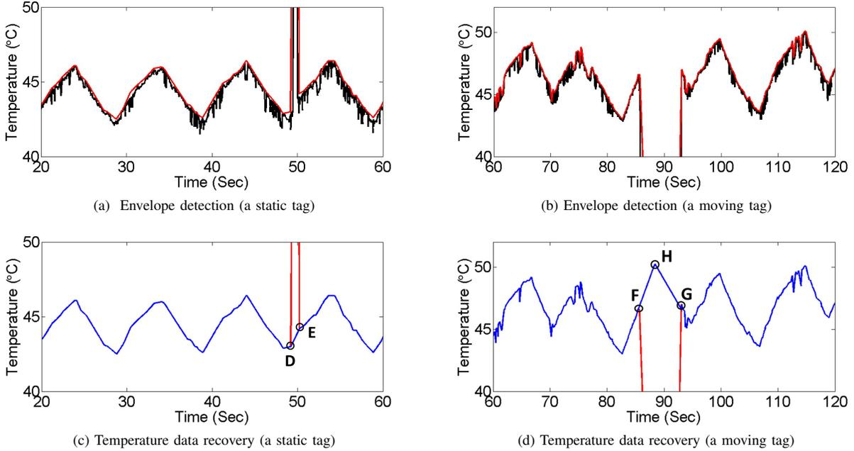
Figure 2: The temperature readings of a static tag or moving tag obtained after applying envelope detection (the upper graphs), and temperature data recovery (the lower graphs). The black lines are the raw temperature data. The red and blue lines indicate the temperature readings after applying envelope detection and temperature data recovery, respectively.
